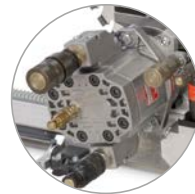
Main motor with leak-oil connection
